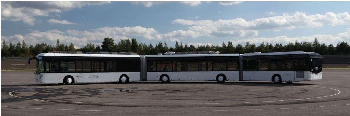
Scientists at the Fraunhofer Institute for Transportation and Infrastructure Systems IVI took up the challenge to make extra-long vehicles maneuverable in city traffic. This was achieved by equipping the vehicle with four steered axles in addition to the fixed main drive axle. A multi-axle steering system, developed and tested at the Fraunhofer IVI, has been implemented in the AutoTram<sup>®</sup> Extra Grand for the first time.
